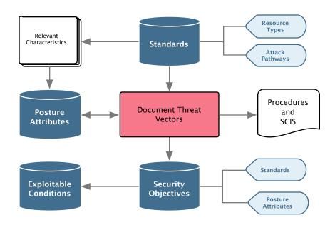
This process is unique to the USM. There is no definition of Threat Vector in any of the NRC developed or endorsed documents. There is a definition for the Attack Pathways, but they alone are insufficient to determine the necessity of the CSP Standards.
