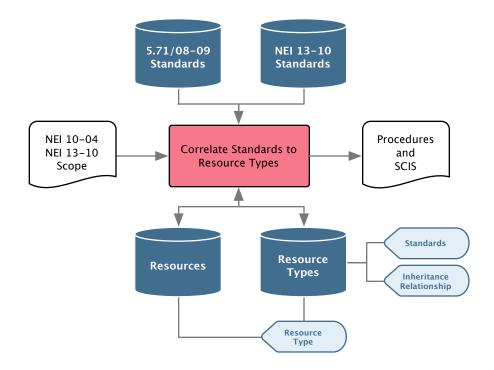
This process starts with the Standards in structured data and results structured data definitions for the Resource Types and Resources.
